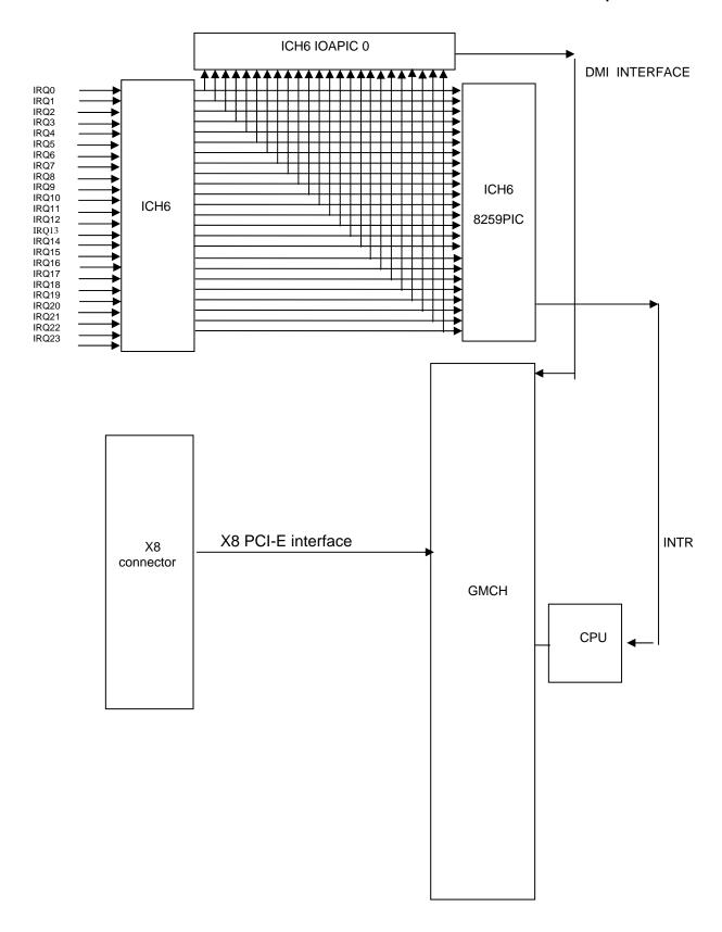
Figure 3. Interrupt Routing Diagram
